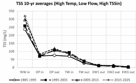
**Fig. 2. TSS change from inlet to outlet (High Temp, Low Flow, High TSSin)**
