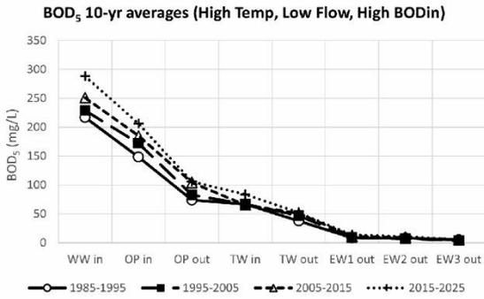
**Fig. 1. BOD<sub>5</sub> change from inlet to outlet (High Temp, Low Flow, High BODin)**
