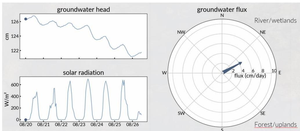
**Fig. 2.** Animated visualization of measured groundwater flux, head and solar radiation
