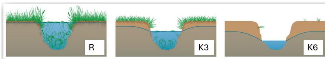
**Fig. 2.** Schematic visualization for three scenarios for mowing the riverbed (R- current state; K3- average mowing; K6- complete mowing)
