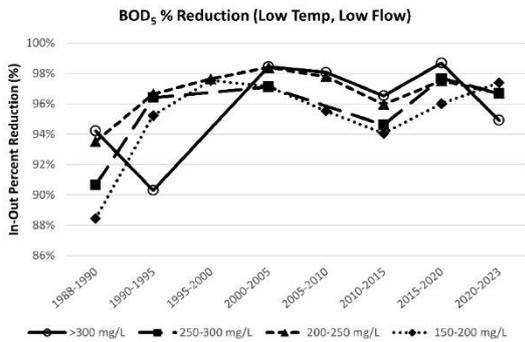
**Fig. 3. Inlet to Outlet BOD<sub>5</sub> percent reduction from 1988 to present (Low Temp, Low Flow)**
