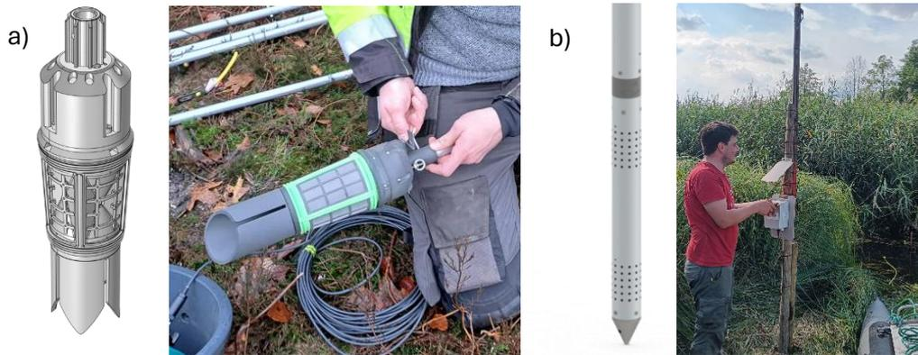
**Fig. 1.** Horizontal (a) and Vertical (b) iFLUX sensor probes, installed at in Stary Rogozyn.
